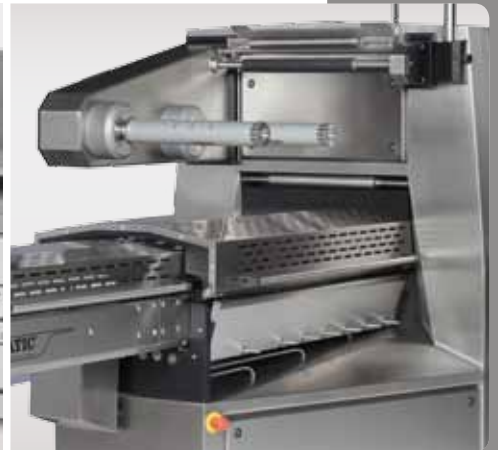
Duplex top film unwinding system for continuous production flow
