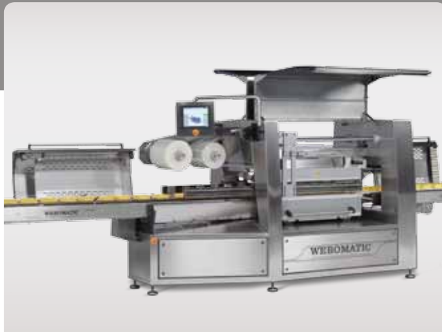
TL 1100 in cleaning position: open design featuring slidable and tiltable covers
