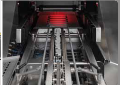
Precise tray positioning by fiber-optics
