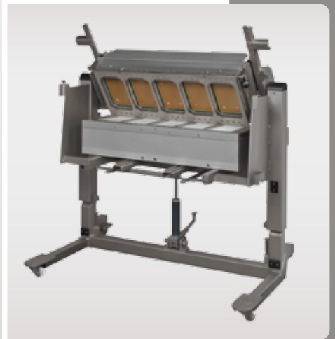
Optional cart for convenient and safe die change
